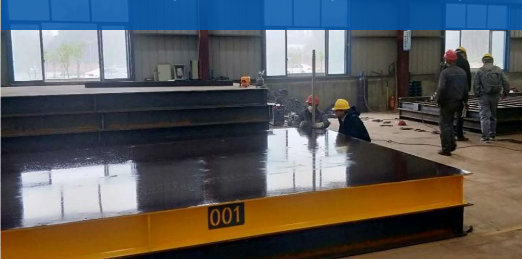
Flatness measurement before the mold table leaves the factory (our Sichuan Vanke project)
