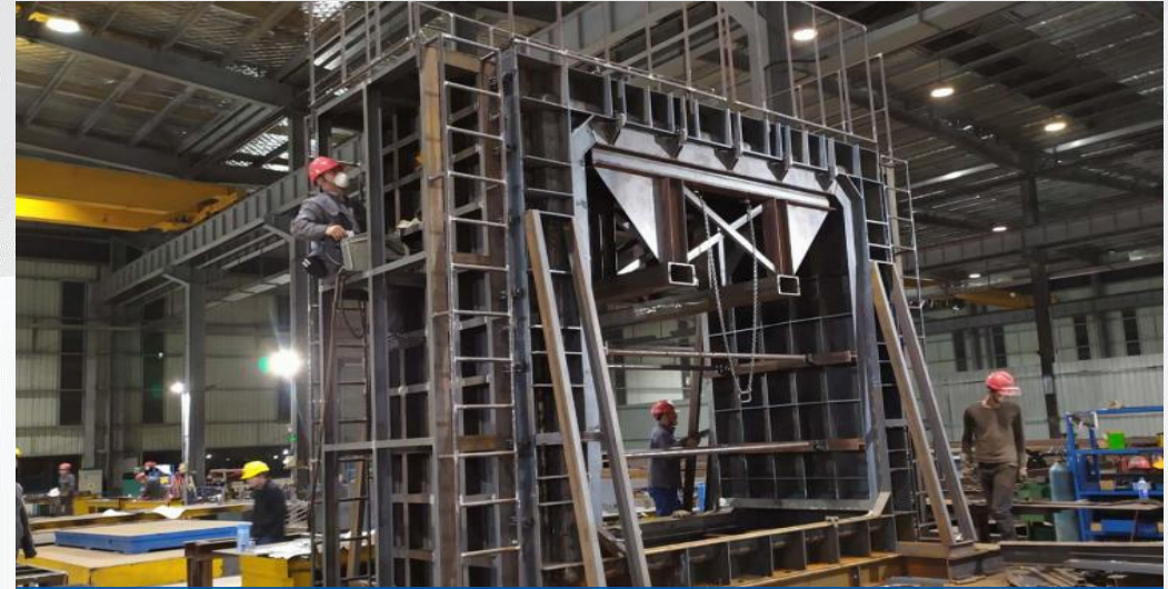
Horizontal pipe gallery mold processing site
