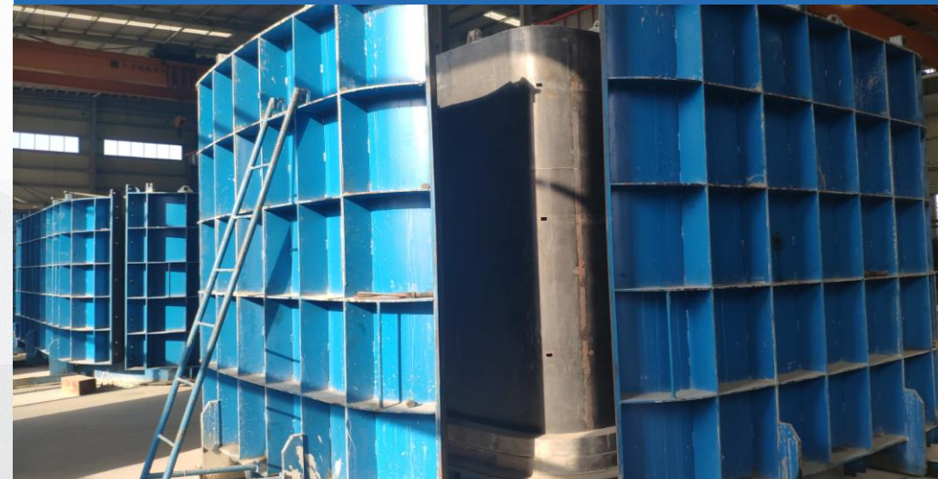
Multi-segment arc pipe gallery mold use site
